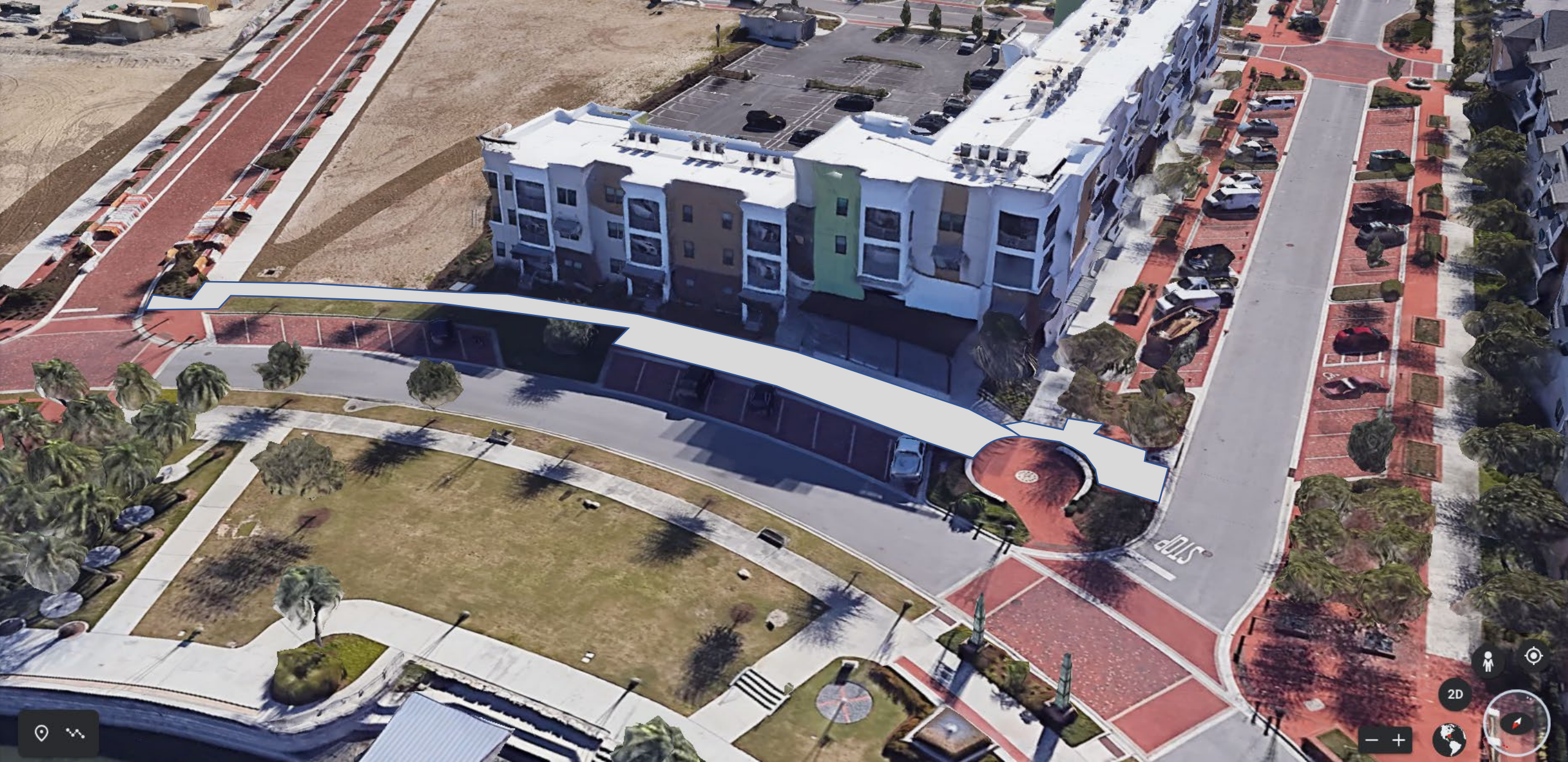
Center Lake Lane corners of City Plaza Way & City Walk Lane Remove existing pavers, replace with concrete keeping paver ribbon around landscape planters.
