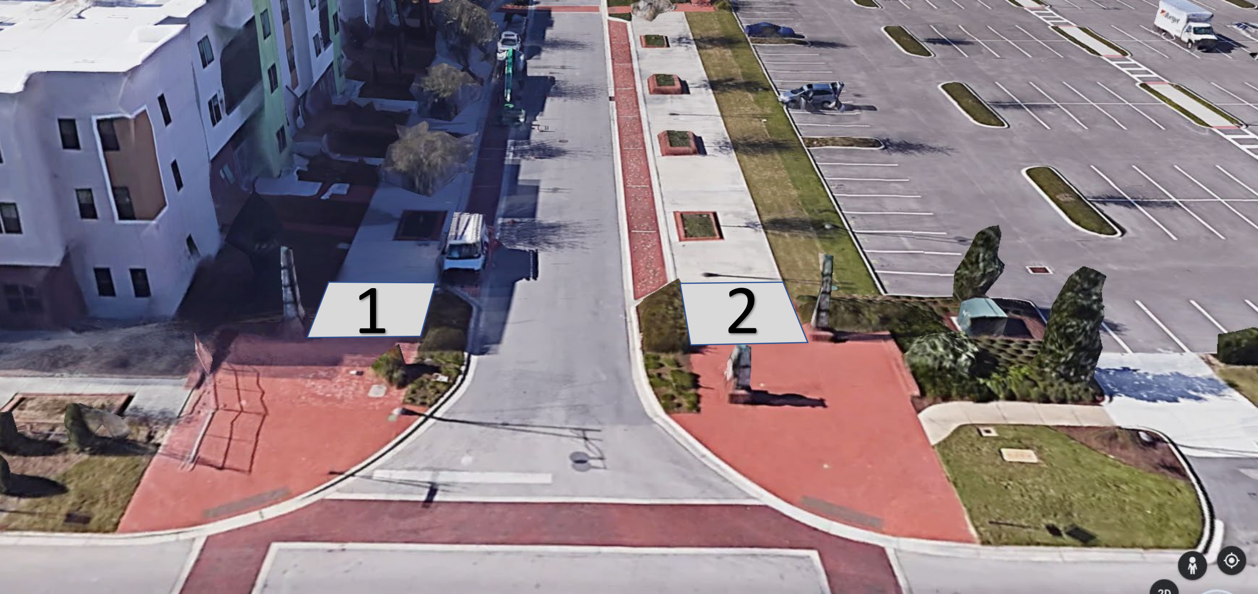
Corner of Oviedo Blvd. & Center Lake Lane Remove existing pavers in areas marked 1 & 2 and replace with concrete.
